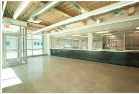
Inside, the redemption center has a modern, industrial look, with polished concrete floors, oxidized metal panels, natural materials, and exposed fireproofing and decking.
